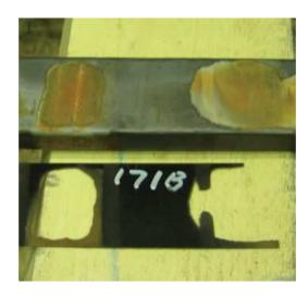
This slot portion of the bars for Unit 4 at Peace Canyon shows erosion of a significant amount of semiconductive coating and side packing. This erosion was caused by PD activity that occurred between the bar surface and slot.
